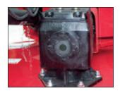
The patented oil sight gauge takes the guess work out of checking the oil. In less than 10 seconds, all three cutting box oil levels can be checked and rechecked as often as you walk around the machine. Never climb onto the cutter again to check the gearbox oil levels.
