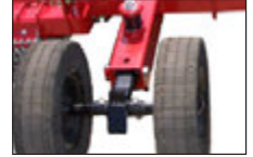
Each axle arm on the center and wings has a spring cushion to absorb the shock loads near the wheel.
